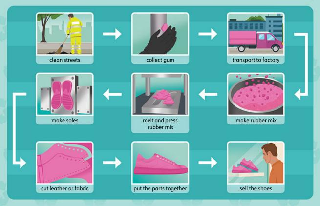
This is how the shoes are made. The streets are cleaned, the gum is collected and transported to a factory. Then the gum is broken down into small pieces and it is added to rubber to make a new rubber mix. The rubber mix is melted and pressed to make the soles of the shoes. Then **leather** or fabric is cut to make the top parts of the shoes. Factory workers put the parts together and then the shoes are ready to be sold in shops.
